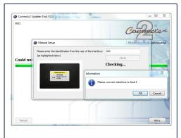
The updater tool will check to see if the correct lead is being used. If the correct lead is being used this will also check the software.
