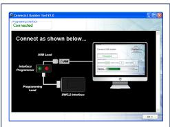
2 Connect the C2 upfater tool to your computer. Use the lead labelled 'PROG LEAD 2' initially. The box in the top left hand corner will show you when the computer has detected the C2 updater tool.
