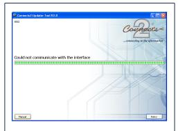
If the message 'Could not communicate with the interface' is displayed, you may need to use the lead labelled 'PROG LEAD 1'. Click 'Manual' if the bottom left corner of the screen.
